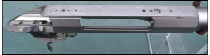
Unlike American rifles, where the recoil lug is located between the barrel and receiver, the Tikka's recoil lug is a groove in the receiver and the actual lug is built into the stock. This is a very Scandinavian design and something I also experienced with the Norwegian Kongsberg rifles. The receiver secures to the stock using the traditional two master screws and the magazine well is again a one size fits all arrangement.
