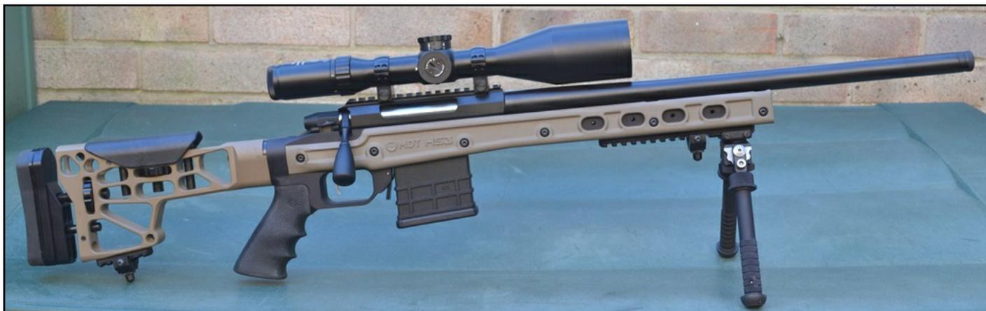
To complete the build, I fitted an Atlas bipod, which in my opinion are one of the best bipod's on the market, scope rings were German 30mm Reznagel which although relatively expensive are of excellent quality and the scope was a German Tactical KAPS 2.5-10x56.
