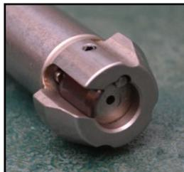
Bolt lift is 60° and like all modern bolt mechanisms the bolts cocking mechanism cocks on opening. The cocking piece protrudes from the rear of the shroud with a red dot when cocked thereby acting as a gun state indicator. Removal of the aluminium shroud and firing pin permits the removal of the bolt handle, making this a fairly simple bolt mechanism that is very easy to strip but with excellent
