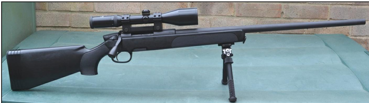
My personal specification for this rifle was to engage targets between 100 & 600 yds, therefore standard rings, picatinny base and a x12 scope was utilised. From a reloading standpoint, this specification dictated that I did not require maximum velocities and therefore using Vihtavouri N150, Lapua brass and scenar 123gr bullets, I loaded 50rds using between 33 and 37.5 grains of N150.
