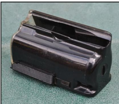
The magazine is retained by two catches either side of the magazine and positioned by a single plunger at the front of the magazine. Feed reliability is superb, regardless of the bolt cycle rate and I have have yet to experience a misfeed.
