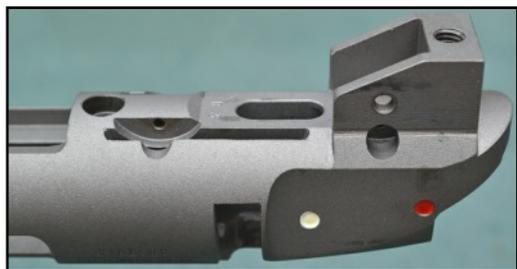
Below the ejection port is the magazine well, which was designed from the outset to work in conjunction with a detachable rotary five round magazine.
