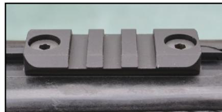
Although I had a set of original Steyr rings I opted for an aftermarket picatinny rail, which permitted the use of Rechnagel tactical one piece mount and the fitting of a S&B 6-12x56 P1 mildot scope.
