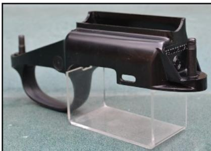
The trigger guard and magazine housing is a one piece assembly and the two master screws pass through the trigger guard assembly securing the stock to the rifle. However a common fault with all plastic trigger guards and the SSG69 is no exception is that the plastic is unable to withstand the crushing force of the screws and will crack easily making this a design weakness.
