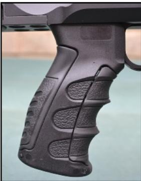
The pistol grip is an ergonomic design and is provided as standard with various front and rear sized panels to accommodate different hand sizes. This is a good idea and something that I have not seen on other designs. The panels can be adjusted by simply removing two pins, remove the panels and assembling in reverse order.
