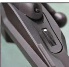
3. Grey plunger; the bolt is locked, cannot be opened and the trigger cannot be depressed. However this position has the added function that the bolt handle can be further depressed, making the rifle easier to transport or store. The manual also states this has added firing pin safety. Once the bolt handle is depressed it can only be released by depressing the grey plunger and rotating the safety to the white indicator.
