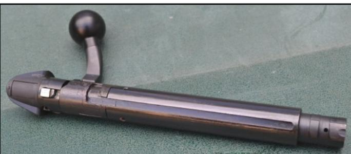
Whilst the principle method of locking is the bolt front locking lugs there is a small lug at the rear of the bolt body that engages in a corresponding lug in the receiver. I am unsure of the lugs purpose other than as a safety lug but I may be wrong.
