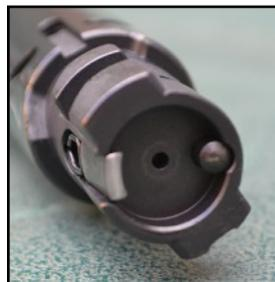
twin front locking lugs and the traditional but very effective spring loaded extractor and a plunger style ejector. The bolt head is integral with the bolt body and when the bolt is rotated, the lugs and the bolt body rotate with only the bolt shroud (sleeve) remaining stationary. In the bolt body there are two grooves, the straight long groove aligns with the cocking bent is where the bolt stop engages. The circular
