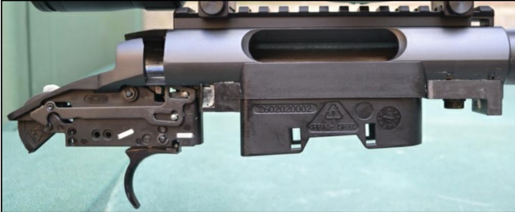
The internal surfaces generally lack the more complicated machine processes found on earlier generation rifles and has only one internal cam face. This is typical of modern manufacturing techniques making the receiver much easier and more cost effective to manufacture.
