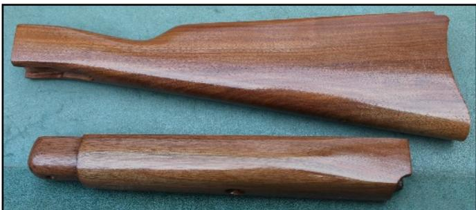
The next task was to restore the woodwork. The woodwork had some minor scratches, the handguard was cracked and different parts of the barrel trough where touching the barrel. As can be seen in the image below, I repaired the cracks, relieved the barrel trough and restored the finish. As the barrel band had the potential to effect accuracy, I
