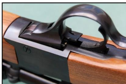
profile forces the user to place two fingers into the cocking lever thereby creating a semi grip configuration and improving handling.
