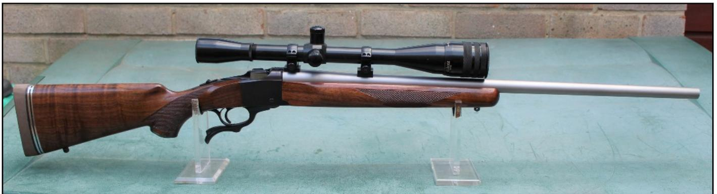
recover that lost two inches. As can be seen in the images, I fitted an adjustable recoil pad, polished the metal components and refinished the butt giving it a more glossy finish. The end result was quiet pleasing, as can be seen above.
