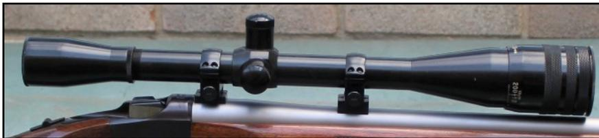
The replacement barrel has a different profile and therefore the quarter rib cannot be swapped onto the replacement barrel. On previous No. 1's I had used Leupold STD rings, however these were out of stock and therefore I decided to fall back on my tried and tested Rechnagel rings, which required the manufacture of a suitable set of bases.
