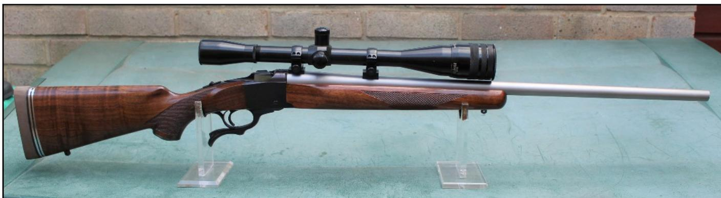
Reloading with 44.5 grains of N140, I zeroed the rifle and achieved an average group size of 22 13 and 12mm, which gave an average grouping of 15 mm. Excellent result and perfectly satisfactory for a rifle of this type.
