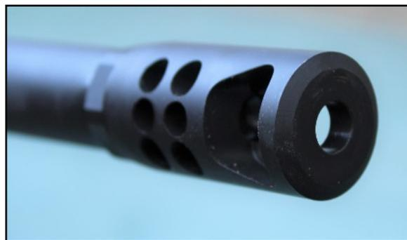
barrel is fitted with an effective steel muzzle brake, which together with its locking nut adds a further 2" to the barrels overall length. As modern factory rifles go, I cannot recall a rifle with such a large barrel. As a long range rifle, not only is this a very efficient as all the propellant burns within the barrel but in the prone position, the whole rifle system is very stable. The heavy weight of the barrel, together with the muzzle break effectively tames the felt recoil.
