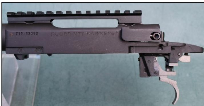
As can be seen in the images, the Hawkeye's receiver is flat sided and this is advantageous when it comes to the receiver/stock fitting. Woodwork can be machined to tight tolerances and this Hawkeye was a good example of a good receiver/stock fit and therefore if standard accuracy is required, then the rifle does not need bedding.
