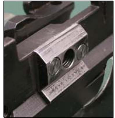
The next process was to black the receiver and pads and then refit, loctiting the screws in place with Loctite 222.
