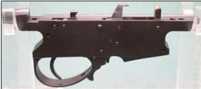
However there were two issues. The trigger is non-adjustable and at some point it had been polished and painted. The original unit was anodised. As you can see from the pictures the paint was easily scratched and simply wiped off if certain oils were applied.
