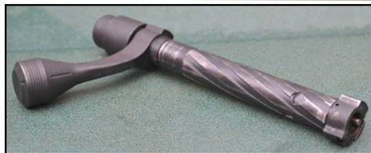
The bolt head is similar in some respect to the savage bolt head. The two lug bolt head has the extractor and ejector built into the bolt face and in turn the head is pinned to the bolt body. This method of securing the bolt head allows some movement between the bolt body and the bolt head which in my opinion allows the bolt head to align slightly with case adding a degree of improved accuracy.
