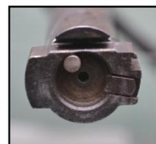
The bolt handle, bolt body and cocking piece shroud have a slightly coarse appearance which gives me the impression they were manufactured as castings. Some people might turn their noses up at this but one must remember this is a budget rifle and although not cosmetically pleasing it does assist in keeping the price of rifle in a more modest bracket.
