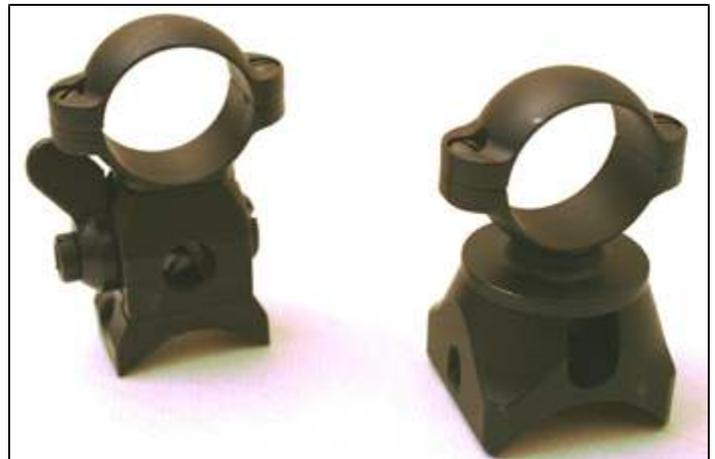
These turret rings have certain other advantages, they have a see-through capability allowing the use of your iron sights, there shear height allows you to fit a scope with the current bolt handle, they have the ability to allow you to remove your scope and refit it without having to re-zero and they have screw adjustment for windage built into the base, ideal for the scope shown below which only has elevation adjustment.
