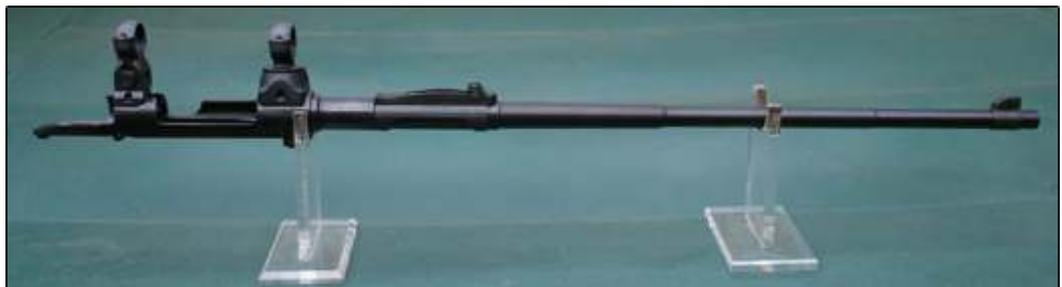
I checked the rifles headspace, firing pin protrusion and cycled some drill rounds through the action to ensure the rifle fed, extracted and ejected correctly. In cycling the action I also checked to ensure the bolt handle cleared the scope, which with classic rifles is something you must be cautious off.
