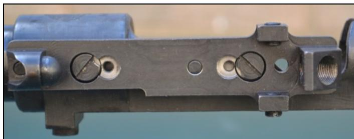
One criticism that I do have with this mount is that the main screws had no recesses to allow the locking screws to engage which amounts to poor quality control and an extra cost for the buyer.
