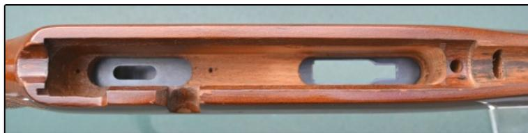
main screw and the barrel does not float as it is designed to sit on the forend. The trigger guard is a simple press steel design, sits on a fascia plate and secures direct to the stock. Butt plate is a simple plastic affair that in this rifle has taken an impact or two, whilst OK if I can find a new or serviceable plate, I will replacement it.
