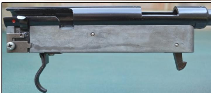
Behind the magazine well is the ejector which is very similar to the Anschutz design and secures in the same manner, although it is a more flimsy design.
