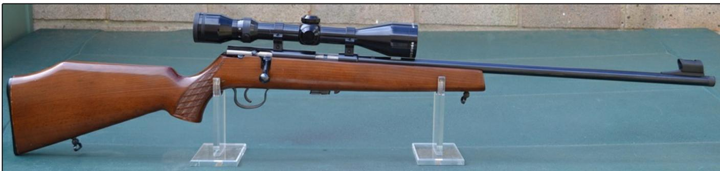
The picture above shows the rifle after stage one, having been completely stripped, cleaned and serviced. I installed a foresight although it was not an original Mauser design, fitted some period sling swivels and applied a temporary scope for the range tests.
