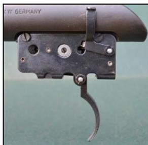
The safety sits on the right hand side and consists of a large thumb plate which has a very positive and long pivotal motion which provides the shooter with an obvious on-off action. When the safety is removed a red peg is shown to indicate the rifle can be discharged, this cant be seen in the dark, however the shoot can feel the recess the peg sits in.
