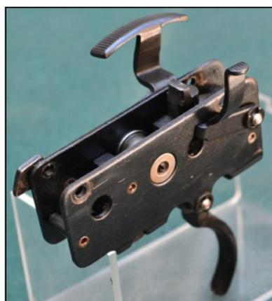
This trigger is a single pull unit releasing at 4.57lbs which was crisp but a little heavy in my opinion and upon inspection there appeared to be no obvious adjustment, which I thought shortcoming to what was otherwise a good trigger unit.
