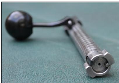
bolt face is recessed with a plunger style ejector and a claw extractor. The bolt body is nicely jewelled as a standard feature.
