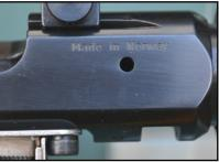
The front of the receiver is threaded to receive the barrel and either side of the receiver are the two largest flats measuring 18.5mm. These two ground surfaces match corresponding surfaces in the stock thereby provid-
