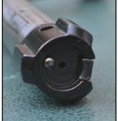
the bolt is disengaged and withdrawn to the rear the lugs runs in there own tracks in the receiver making the action extremely smooth with very little bolt slop when the bolt is fully extended.
