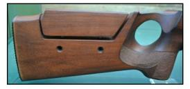
appearance. The layout of the pistol grip creates a deep butt assembly which has an adjustable cheek piece whose height is controlled by two large grub screws threaded directly into the walnut stock. The butt pad is a simple plastic plate that is glued into
