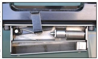
zine has a spring loaded gate, controlled by a lever as shown above. Each time a new round is inserted into the magazine the gate is pushed to one side, reasserts itself and holds the round in place. If the rounds require removing the lever is depressed which depresses the gate and the rounds are ejected from the magazine under the influence of the magazine platform and its spring.
