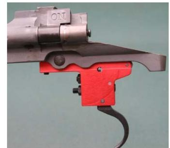
Once fitted and for the purpose of safety you should always test cycle the bolt and ensure the trigger cannot release the firing pin.
