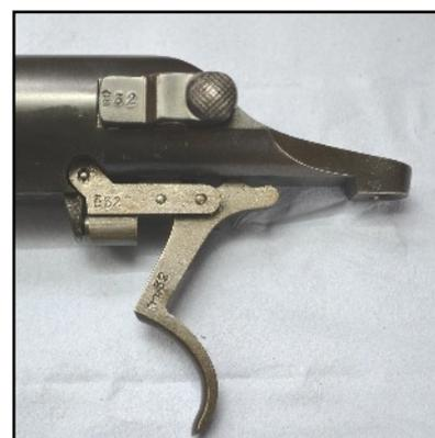
The trigger is a simple and very effective design, consisting of only three major parts, the trigger, sear and trigger spring. As with many trigger systems of the time, the first and second pull is obtained by two cams situated at the top of the trigger.
