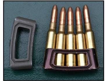
As charger clips are quiet expensive, fairly rare and essential to the carbine's effective operation, the clip should be treated with care. Loading the clip correctly is important. The three inner cartridge seat flush and to the rear, touching the clip. The two outer cartridges and their rims, seat forward of the three inner cartridges.
