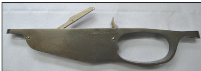
The charger clip catch holds and positions the clip and releases the clip when the rifle needs to be emptied. The elevator doesn't touch the charger clip at all, if you place an empty clip into the mechanism it would pass all the way through. The elevator arm places pressure on the bottom cartridge in the clip and then that spring pressure is transferred through the five cartridges until it is passed into the clip through its lips.
