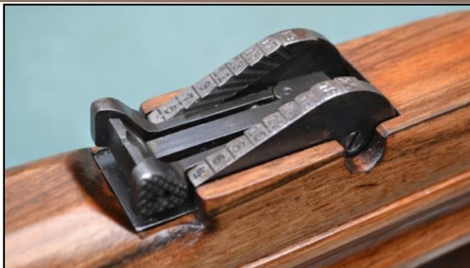
One minor criticism at this point concerning the carbine sights. The sight picture is poor with the sights set at the minimum range of 300. This is due to the combination of the foresight blade being too thick and the rearsight V notch is too small. Re-profiling the foresight blade, would reduce this problem.
