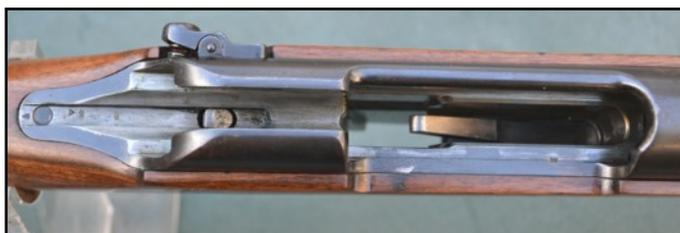
receiver is designed to work with a charging clip as an integral part of the mechanism and therefore, there is no internal magazine as can be found on the Mauser for example. To help the reader understand more clearly how the receiver design assists the rifle's function, it may be prudent to describe the charger clip system.
