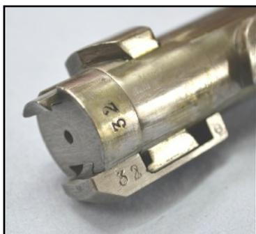
ejector in the bolt head. As the bolt is withdrawn to the rear, the floating ejector strikes the bolt stop, is forced forward and therefore pivots the empty case on the extractor and away from the rifle.
