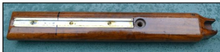
Once repaired, the forend had to be cut to length, providing the correct handling, the correct size in relationship to the new barrel length and the correct profile.
