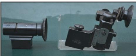
The rear aperture sight was a Parker Hale PH25B and was secured using a receiver side rail. A traditional block was used for the foresight assembly and a further two blocks were fitted along the barrel, should the user wish to fit a scope.
