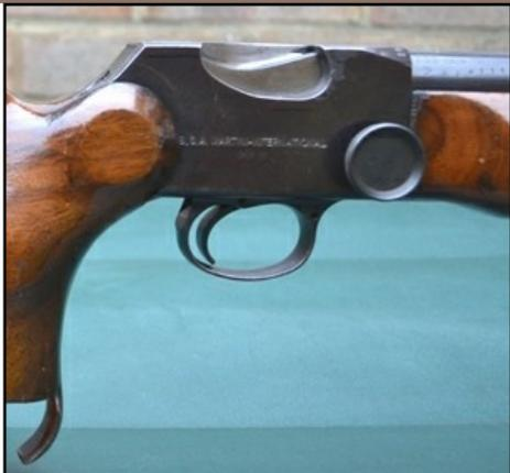
The BSA MkII came originally in two types, a heavy & light barrel version. The rifles overall length is roughly 44.0", with a barrel length of 28.0", weight was a hefty 14.0lb and rifling was six groove with a 1 in 16" twist.
