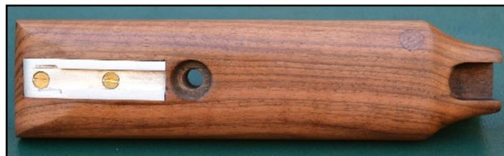
The old accessory rail had to be stripped, cleaned up and refitted, filling in any gaps that were left from the amateur fitting.
