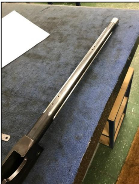
As the rifle was going to be used for field work, a moderator was required and therefore the muzzle was threaded for a moderator and fitted with a flush fitting thread protector.
