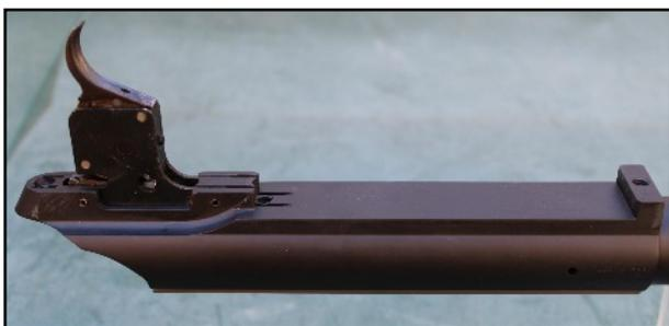
The lower receiver is secured to the stock via the traditional master screws and a single recoil lug. The bottom of the receiver is flat for an accurate and strong receiver to stock bond. The lack of a magazine well adds to the rigidity of the receiver design and therefore increases accuracy. To the rear of the receiver is the trigger assembly well, where the one piece trigger unit is secured using two pins.
