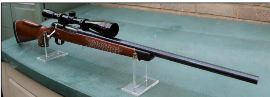
The seller was supportive and I got the rifle relatively cheap which helped. Once I received the rifle, I stripped it down and cleaned and checked the rifles condition. Despite the worn barrel, the action was sound, the ejector was rusty and therefore wasn't working efficiently and the stock was showing signs of wear of a typically well used thirty year old rifle, however all, was easily repairable.
