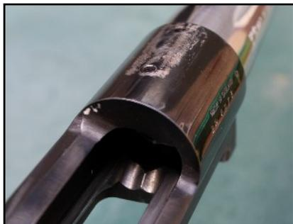
.222 Remington, the loading/ejection port is a shade over 3¼" which accommodates calibres up to .308 Winchester. Unlike the CFT discussed in my previous Armourers Report, the upper receiver does not have a 17mm scope rail machine into the receiver, but instead it is drilled and tapped for two scope bases. This is advantageous, as it permits scope bases suitable for other international markets to be fitted, thus making the rifle more attractive, which was essential for the likes of the US market.
