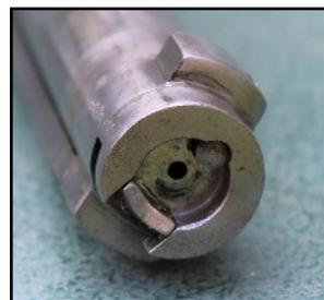
As previously mentioned in the receiver section, a unique feature to the CFT and CF2 was the introduction of the bolt rib, which runs along the entire length of the bolt. The purpose of this rib is to act as a guide and prevents bolt wobble which was common in Mauser type designs.
