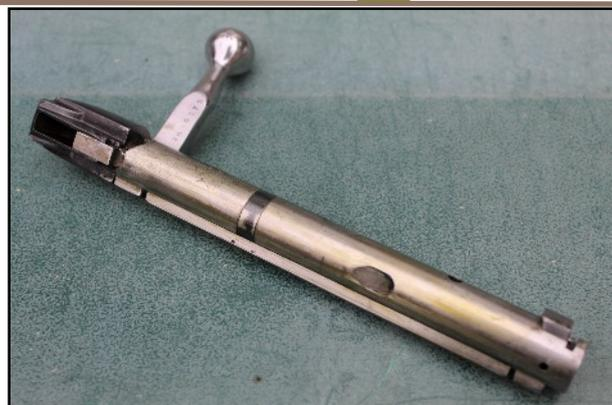
Having overcome primary extraction and the firing pin has been withdrawn, the empty case is extracted from the chamber and is held on the bolt face by the extractor. The bolt face ejector is kept depressed until the empty case clears the ejection port. At this point, it is allowed to raise under the influence of its spring, push the rim of the cartridge, pivot it around the extractor and eject the empty case away from the rifle.
