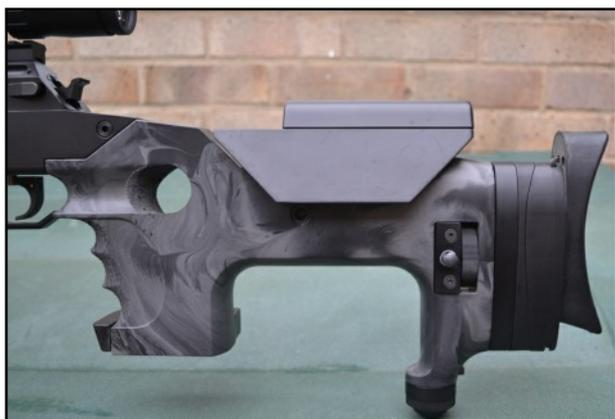
The Alpine butt assembly is an ergonomic synthetic resin moulded butt and pistol grip assembly called CrossTech. It is manufactured by Marti in Switzerland, is completely detachable by slackening one hex bolt and is available in a variety of colours.
