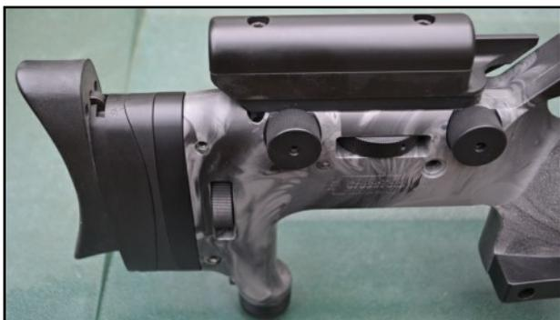
The cheek pad can be removed if required and the cheek pad assembly can be raised and lowered without the need for tools. The butt plate on the other hand can be adjusted for tilt, vertical, lateral and length but adjustment requires a hex key.
