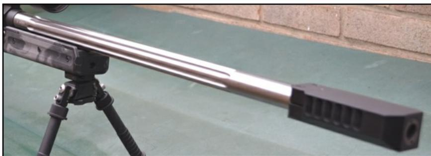
The barrel screws into a bushing which permits the barrels interchangeability as it is the bushing that secures to the receiver and can be removed with relative ease. On this model the barrel retains its natural stainless steel finish but if the rifle was to be used in a tactical role then the barrel would require black cerakoting.
