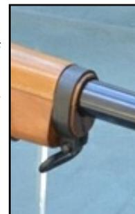
The only upper handguard that I had that was close to fitting was from an old Kongsberg M59A1. However even that was too small and required a further 3mm of height to clear the barrel. To do this I ordered a 5mm sheet of beech and super glued it onto the base of the forend and then machined it all down to 3mm.
