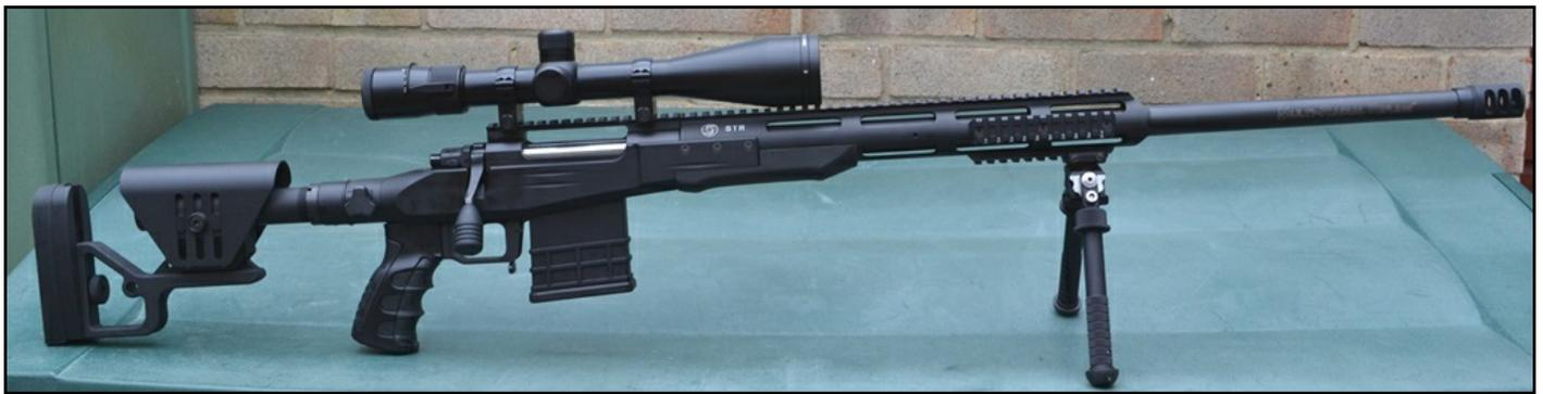
firearm that targets the “tactical” gap in the civilian shooting market and should not be confused with military spec tactical or sniper rifles. The receiver and bolt mechanism is based on Sabatti’s Rover model and the rifle differs from its Mk1 version, with the introduction of a tactical bolt handle, MDT 10rd magazine and a UDP AR style pistol grip.
