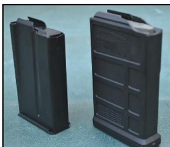
The first replacement magazine was a polymer Magpul AICS compatible 10rd .308 magazine. Testing it with 10 rounds it fitted and cycled 10 rounds without fault. It didn't swell when fully “bombed up” and was actually easier to hand load than the MDT.
