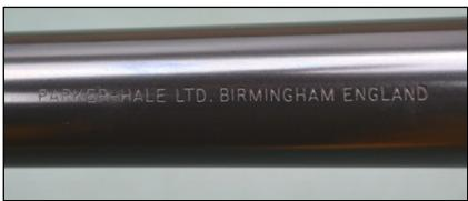
The barrel is not floating but is designed too be supported by approximately 2" of the forend, the finish is a good quality deep blue and is stamped with the words "Parker Hale Ltd, Birmingham, England. The bore is in excellent condition, has four grooves and the rifling has a twist rate of 1 in 12.
