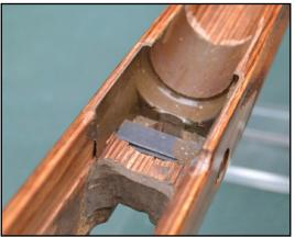
receiver is not bedded and the barrel rests on the forend which does not necessarily reduce accuracy. My only minor criticism is the yellow tint and the poor fitting of the recoil block. The two locking rings do not sit central in their recesses and as a result over the years as the rifle has recoiled and has caused the wood around one of the locking rinks to fracture.
