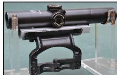
As mentioned previously, the French bracket has a round base, therefore the adaptor is machined from a solid round aluminium bar of the same diameter. The scope is mounted and secured using the same fittings and screws as used on the H&K mount. The only adaptation required to the bracket is the addition of two screws to mount the adaptor.
