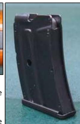
One last point, magazines are integral to the efficient functioning of the rifle and therefore they must be kept clean at all times. When stripping this magazine make note of how the platform comes out as it must go back in the same manner. Failure to reinstall the platform correctly will reduce the magazines round capacity to four and it will struggle to feed the last round.
