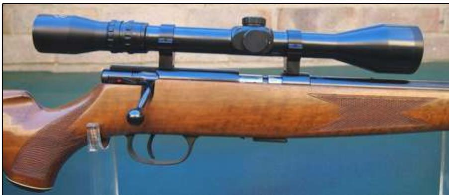
In my scope collection I had a Pecar 4-10 variable. This is a superb 1970/80's scope designed for fullbore rifles of the period and the British Police used it on the Lee Enfield Enforcer as their Sniper Rifle. It has a 25mm tube and a 44mm object lens and would not
