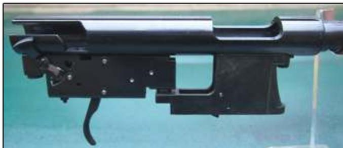
The safety catch is located at the rear and on the right hand side of the receiver, it is easy to operate and has a positive motion when applied or released. The safety catch can only be applied when the bolt is cocked and the application of the safety locks the trigger and prevents the sear from being released, however the bolt can still be functioned and therefore the rifle can still be cleared and made safe.
