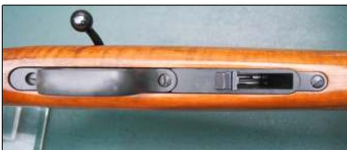
As the rifle is some 12-15 years old the sling swivels are somewhat dated and whilst the barrel is not floating it touches the woodwork ever so slightly. Therefore I replaced the sling swivels with modern QD studs and then fixed a small wooden insert into the barrel channel so the barrels contact with the fore end was constant rather than intermittent.
