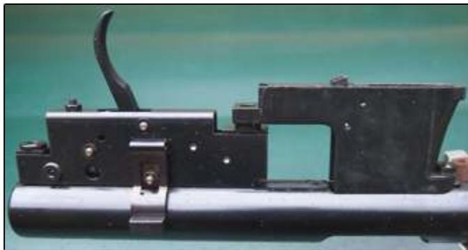
Clearly shown in the picture is a square recess, formed between the trigger and the magazine housing, this provides access to the screw which secures the ejector.
