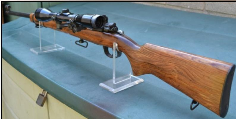
This approach projects the scopes some 3.3" out to the left, which looks odd to most shooters as there is no obvious cheek weld and causes the rifle to be unbalanced as shown in the image to the left. As this section is to discuss the receiver, I will discuss the scope configuration in its own section.
