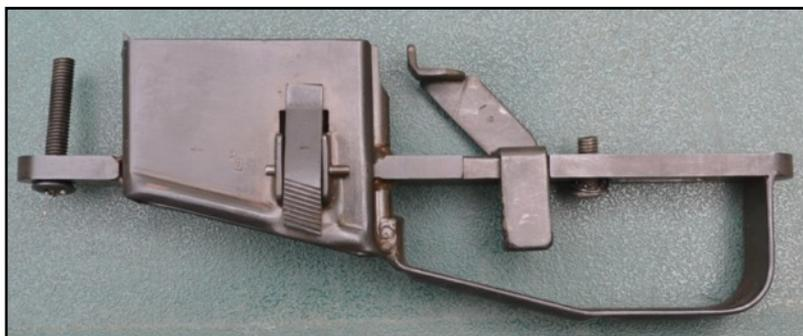
When assembled, the safety catch is located forward of the trigger. The safety catch profile is that of a cylindrical drum welded to a plate, which when pulled to the rear engages with the sear block, locking the trigger mechanism and the bolt. When pushed forward it realises the sear block therefore allowing it to rotate and lowering the sear. Detent action for the
