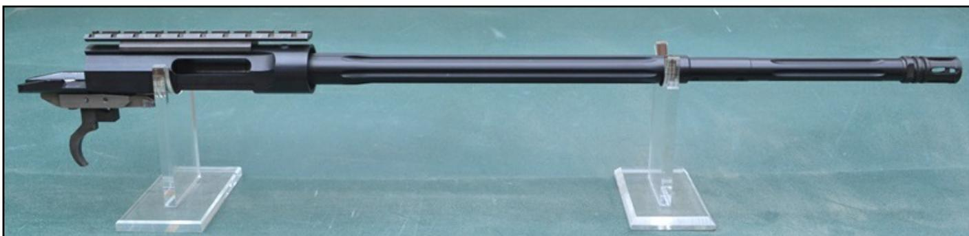
DPMS and has a twist rate of 1 in 8, which permits bullet weights up to 70grn. Although this twist rate can accommodate heavier bullets, bullet weight is limited by the magazine. As this is a AR15/M16 spec barrel, it assembles to the receiver in exactly the same manner as the traditional AR15 and the bolt and barrel lock using exactly the same method, making this rifle very attractive and cost effective to countries already using that rifle system.
