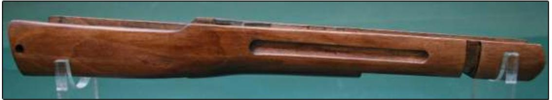
To make the stock fit you have to machine out the wood to accept the M10's receiver, the finger grooves have to be machined as these are absent on the No4 and the stock cut to length. I actually cut mine slightly shorter as I was fitting a telescopic T8 Moderator but there was only a inch difference.
