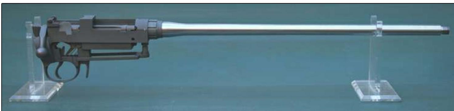
The previous picture above shows the new barrel, same length but a slightly larger diameter across its full length where the original barrel was tapered with the muzzle being crowned and threaded.
